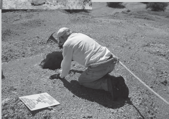
Figure 2: Smith uses a pickaxe to chip away at an underground mine. A rope is tied around his waist in the event that the ground would give away causing him to plunge down a five foot wide shaft.
