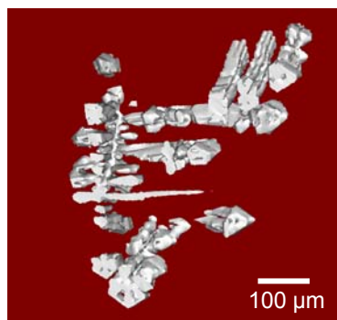
Fig. 2 Three-dimensional (3D) microstructure reconstructed from serial sections, highlighting the complex dendritic morphology of the \text{LaSn}_3
